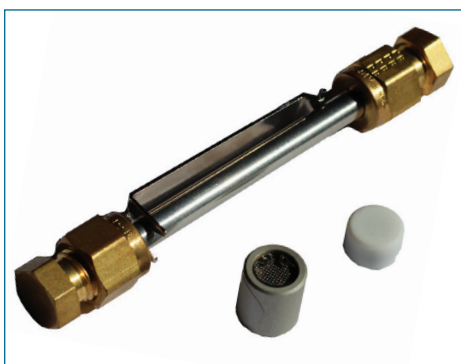
Figure 7. A diffusion pen, worn by a practitioner, can be used to monitor air in the breathing zone
